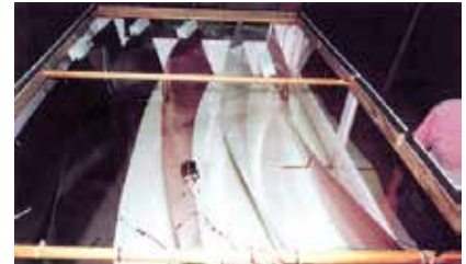
Protected sheet metal test panels and unprotected control panels are scribed and exposed to 800 hours of humidity @ 95°F.
