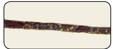
Close-up (25X) of scribe (scratch) PROTECTED by the Final Coat Module.
